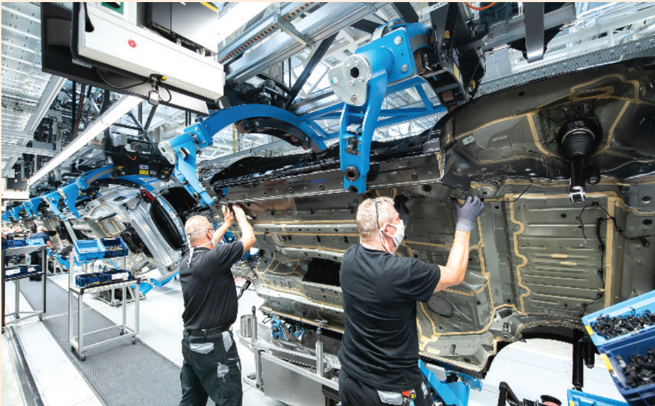
Mercedes-Benz employees lay brake lines on an S-Class at the “Factory 56” plant in German city of Sindelfingen. The luxury carmaker plans to go all-electric by 2030. The transition will necessitate massive changes to the brand’s current lineup of mostly combustion-powered vehicles
