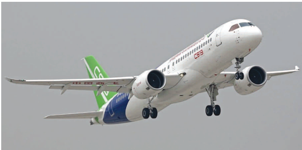
The C919 has a range of 3,450 miles, and can seat up to 168 passengers. This falls short on both capacity and range when compared to rival Airbus’ A320 and Boeing’s 737 Max
