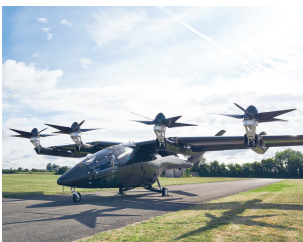
The VX4 electric vertical take-off and landing vehicle rose in a so-called tethered hover test, in which the aircraft was still attached to the ground for safety while its eight propellers pushed it upward
